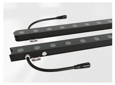
LW01 is designed to provide high quality illumination for columns and architectonic surfaces, with a variety of lens options that can be used for flood lighting, wall grazing, wall washing and accent lighting. With 24VDC input, one constant voltage power supply can load 7 meters in continuous length without brightness degradation from start to end.
