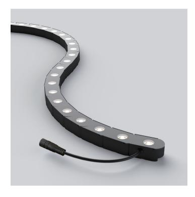
AW01 is designed to provide high quality illumination for columns and curved architectonic surfaces, with a variety of lens options that can be used for flood lighting, wall grazing, wall washing and accent lighting. Equipped with 18 pcs rotatable and waterproof high-power module, it is flexible in horizontal way. With 24VDC input, one constant voltage power supply can load 7 meters in continuous length without brightness degradation from start to end.
