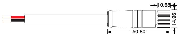
Female Connector M12-F-2C-18AWG-D6-W-0327-S
