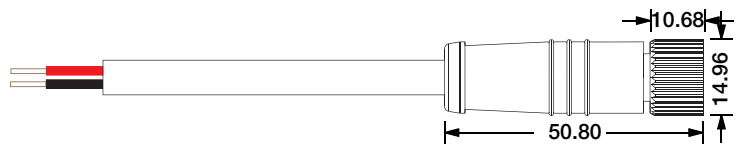
Female Connector M12-F-2C-18AWG-D6-W-0327-S
