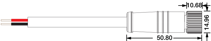
Female Connector M12-F-2C-18AWG-D6-W-0327-S
